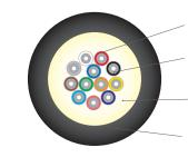
900µm Tight Buffered Optical Fiber
