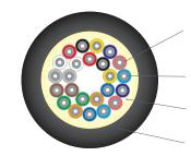
900µm Tight Buffered Optical Fiber
